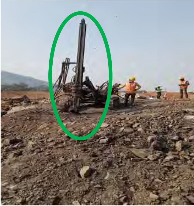
Water sprinkling system provided in Rock Drilling Machine (ROC ) to suppress Dust Emission
